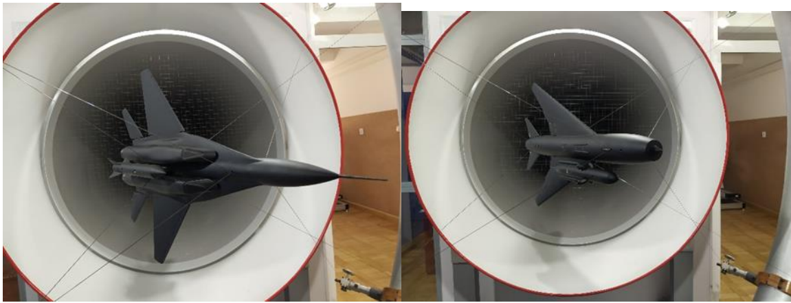
Fig. 11. Wind tunnel investigations of the aircraft-rocket sets (MiG-29 left, Su-22 right)
