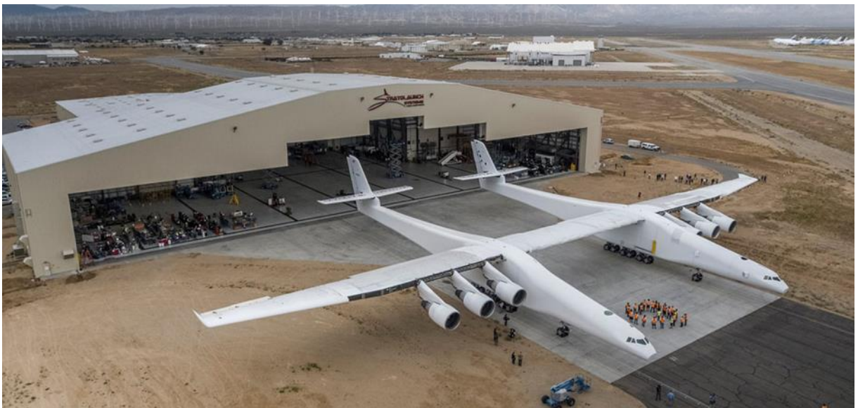
Fig. 5. Twin-fuselage Stratolaunch airborne-carrier during roll out ceremony in 2015
