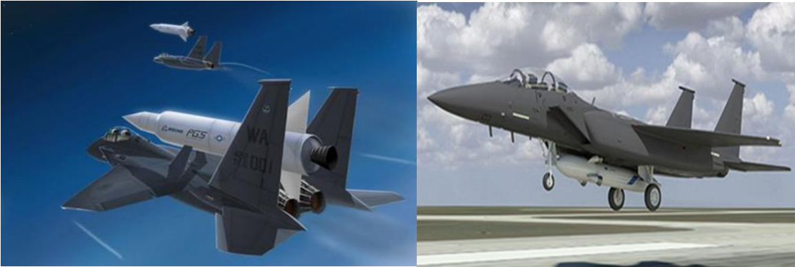
Fig. 6. Evolution of Boeing's aircraft - rocket configurations, left: F-15 Global Strike Eagle with rocket on fuselage, right: F-15E ALASA with rocket under fuselage
